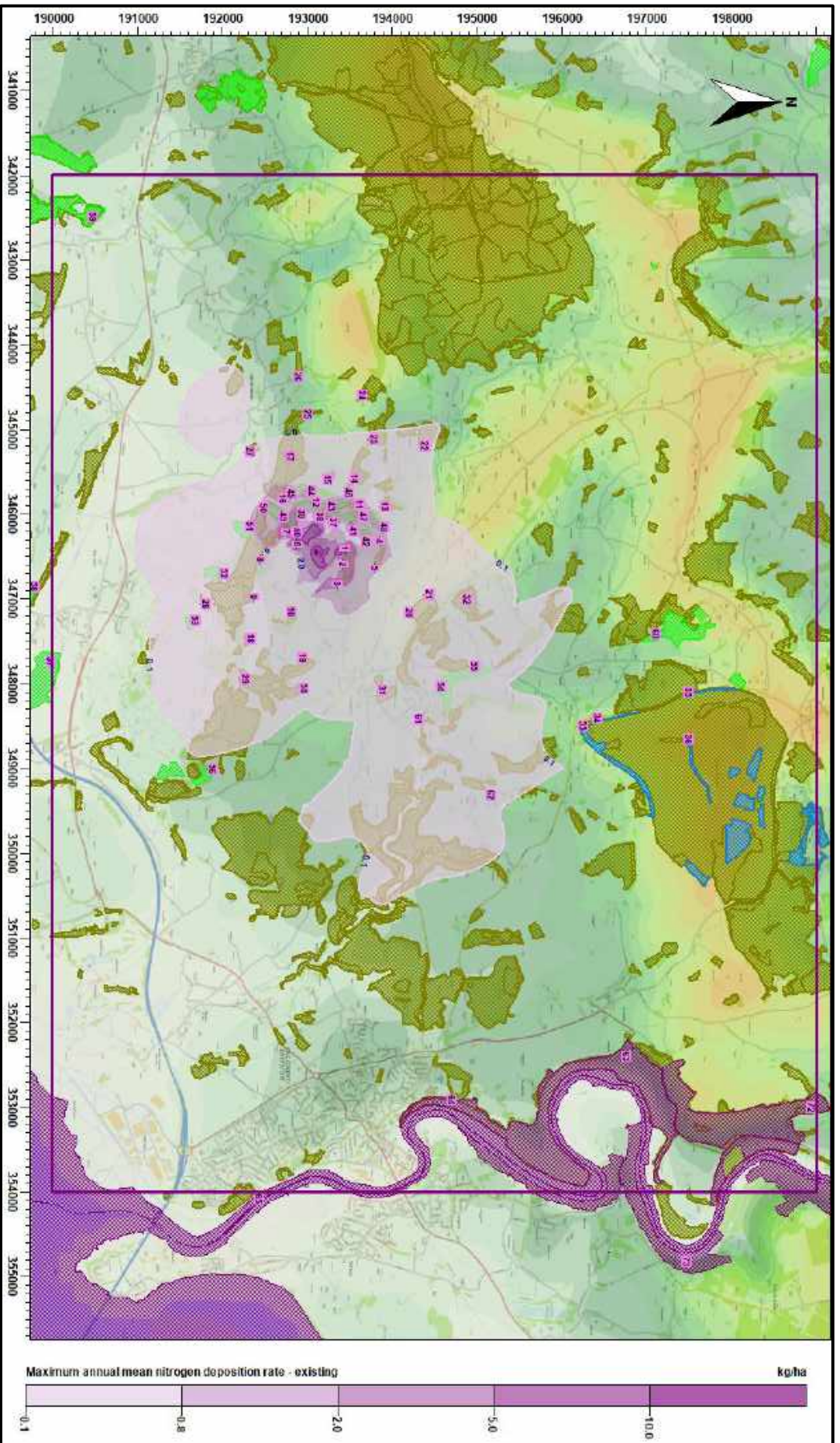
Figure 6b. Process contribution to maximum annual mean nitrogen deposition rate – existing poultry houses
